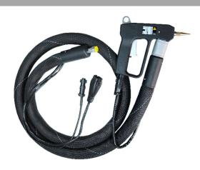
OGAN GN Series Handguns are developed for increasing flexibility of adhesive applications and ease the usage. OGAN GN Series handguns provide constant operational temperature up to 210°C, which guarantees continuous adhesive flow. These hand held compact guns are designed to endure the roughest working conditions, their durable external and internal components provide long service life.
