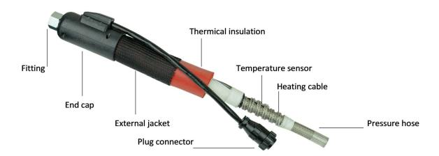
The **pressure hose** is chosen depending on the working pressure, temperature and medium output required. We mainly use PTFE hose in stainless steel braid. The material of this hose features outstanding chemical and temperature resistance (up to 250°C), and very low coefficient of friction. PTFE hoses with strong mesh technology are being used to safely transfer the heated products up to 500 bar.
